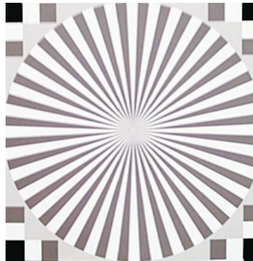
Logitech designs, tests, and refines ConferenceCam optics to optimize image quality factors such as sharpness, distortion, tone reproduction, color accuracy and dynamic range. Test patterns (like the Siemens Star shown here) are used for calibration, alignment, and troubleshooting the signal path as well as fine-tuning corner-to-corner sharpness
