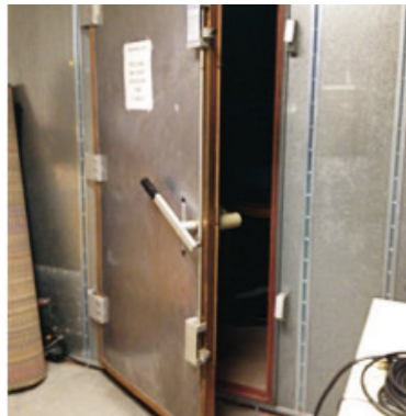
Beyond the door to this EMC chamber, Logitech performs tests to ensure compliance with international electromagnetic emission standards.
