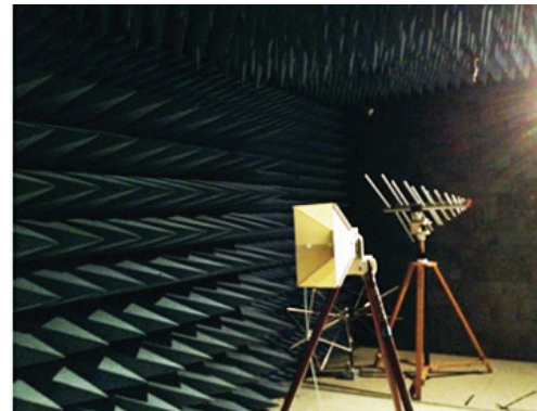
Beyond the door to this EMC chamber, Logitech performs tests to ensure compliance with international electromagnetic emission standards.
