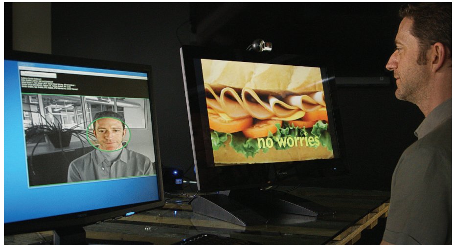
Figure 2. Configure the software to play an advertisement targeting men when the audience in front of the digital sign is male.
